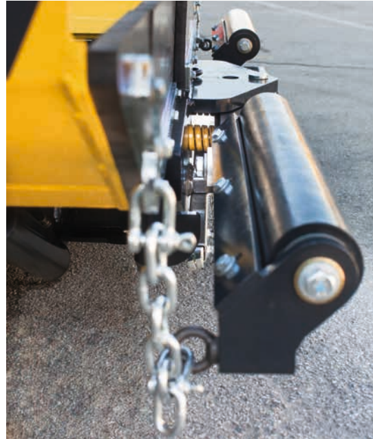
Impact-free docking – dampened bumper.
