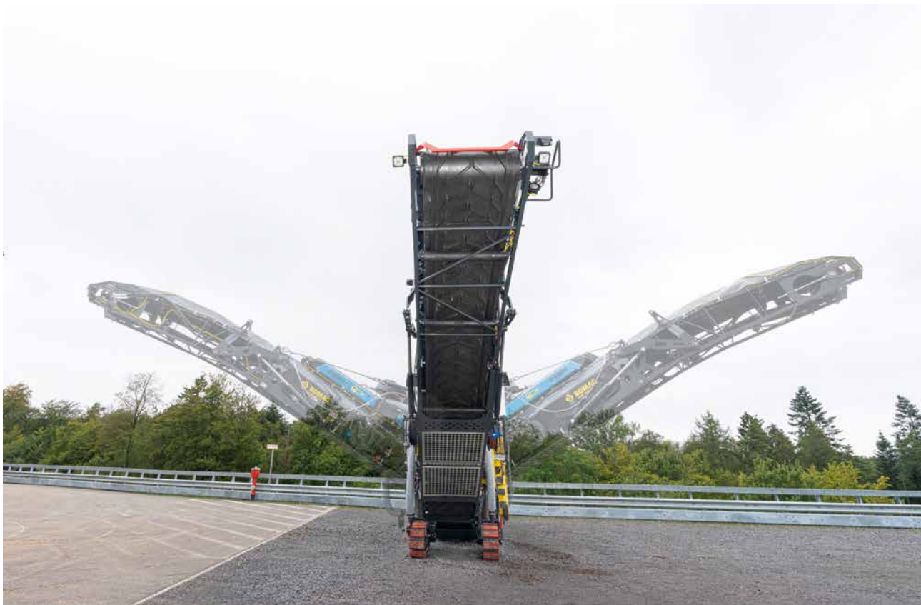
The 130° slewing angle of the conveyor belt ensures maximum manoeuvrability and flexibility when loading the truck.
