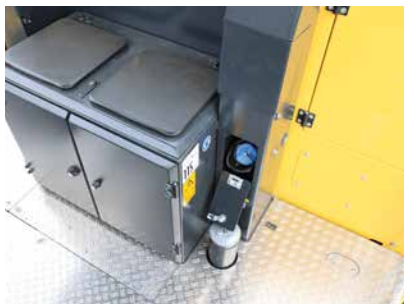
Easy and safe access for refilling AdBlue on the driver's platform.
