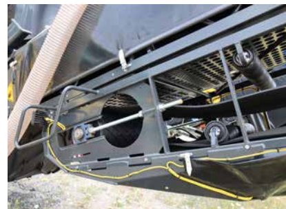
Easy maintenance of the conveyor belt: the drive can be removed for maintenance without major dismantling.
