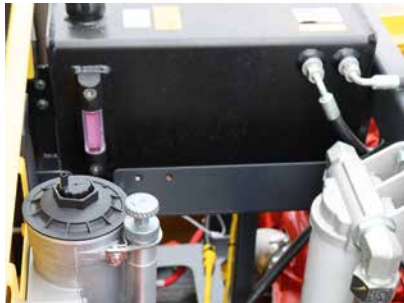
All fluid tanks are equipped with a level indicator that immediately catches the eye.
