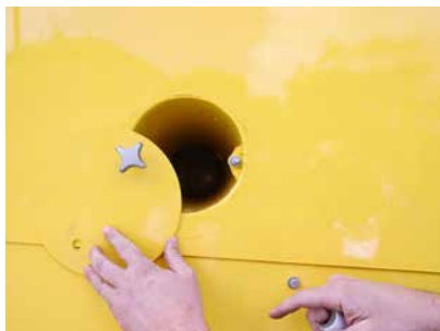
The dust extraction system inside the machine is easily accessible for cleaning, ensuring proper operation.
