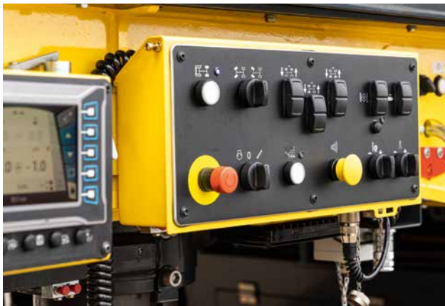
Top equipment for the second operator: operating console and additional display on the ground control panel.
