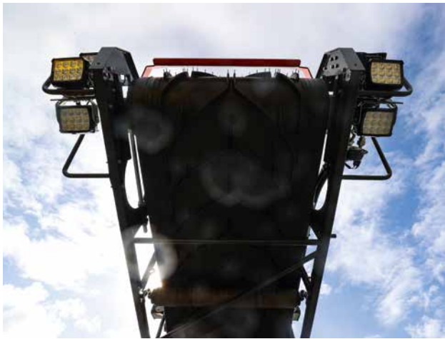
With the additional lighting of the Advanced Night Package on the discharge belt, the trough is perfectly illuminated.
