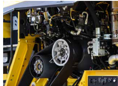
The transmission, hydraulics and engine are within easy reach through wide-opening maintenance flaps on the side.
