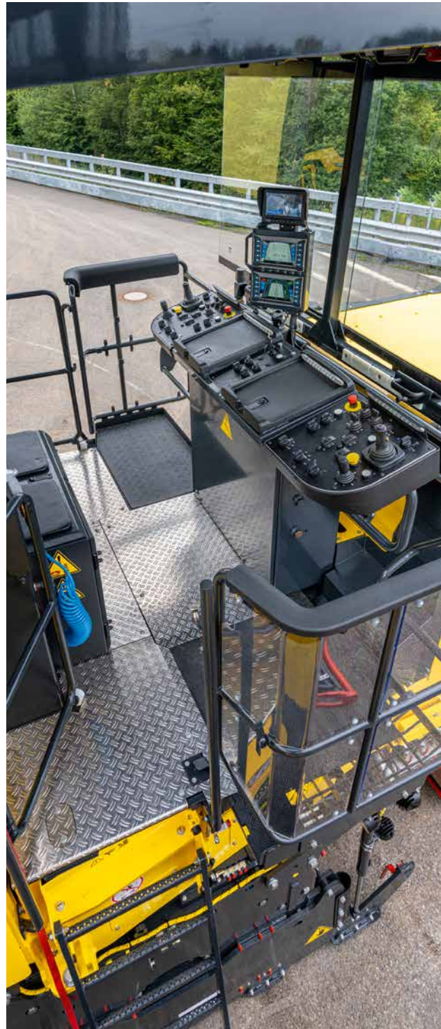
Developed for a clearer overview and intuitive work processes: the driver's stand with swivelling main operating console.
