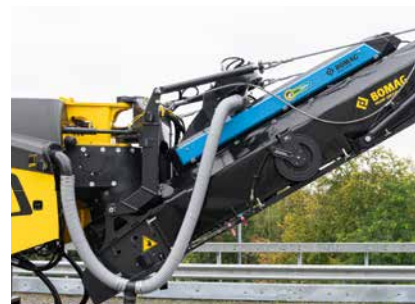
Ingeniously simple, BOMAG's ION DUST SHIELD provides effective fine dust reduction without a filter.
