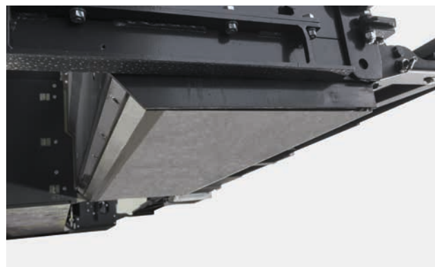
Very long screed plates for perfect asphalt evenness.
