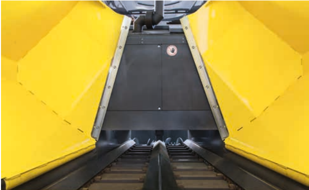
Smooth material flow: the reversible conveyor belt.
