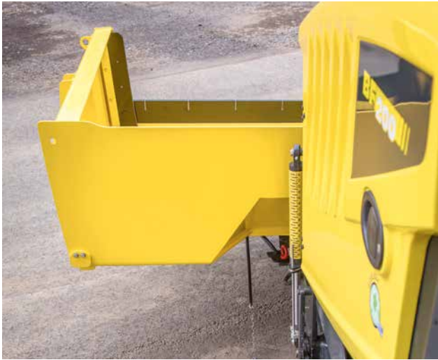
This is thanks to the viewing tunnel which allows a full view of the track drive and dipstick.
